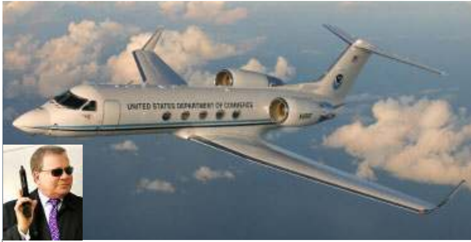
The Gulfstream IV-SP (G-IV) is a high altitude, high speed, twin-turboprop jet aircraft acquired by AOC in 1996. The G-IV is currently configured for operational support of the National Hurricane Center synoptic surveillance mission/ http://www.nasa.gov/images/content/117378main_gulfstream_aircraft.jpg
